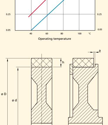
lining does not become cold before it sits properly on the core. Rapid or uneven cooling should be avoided at all costs, as otherwise stresses will form in the lining.
